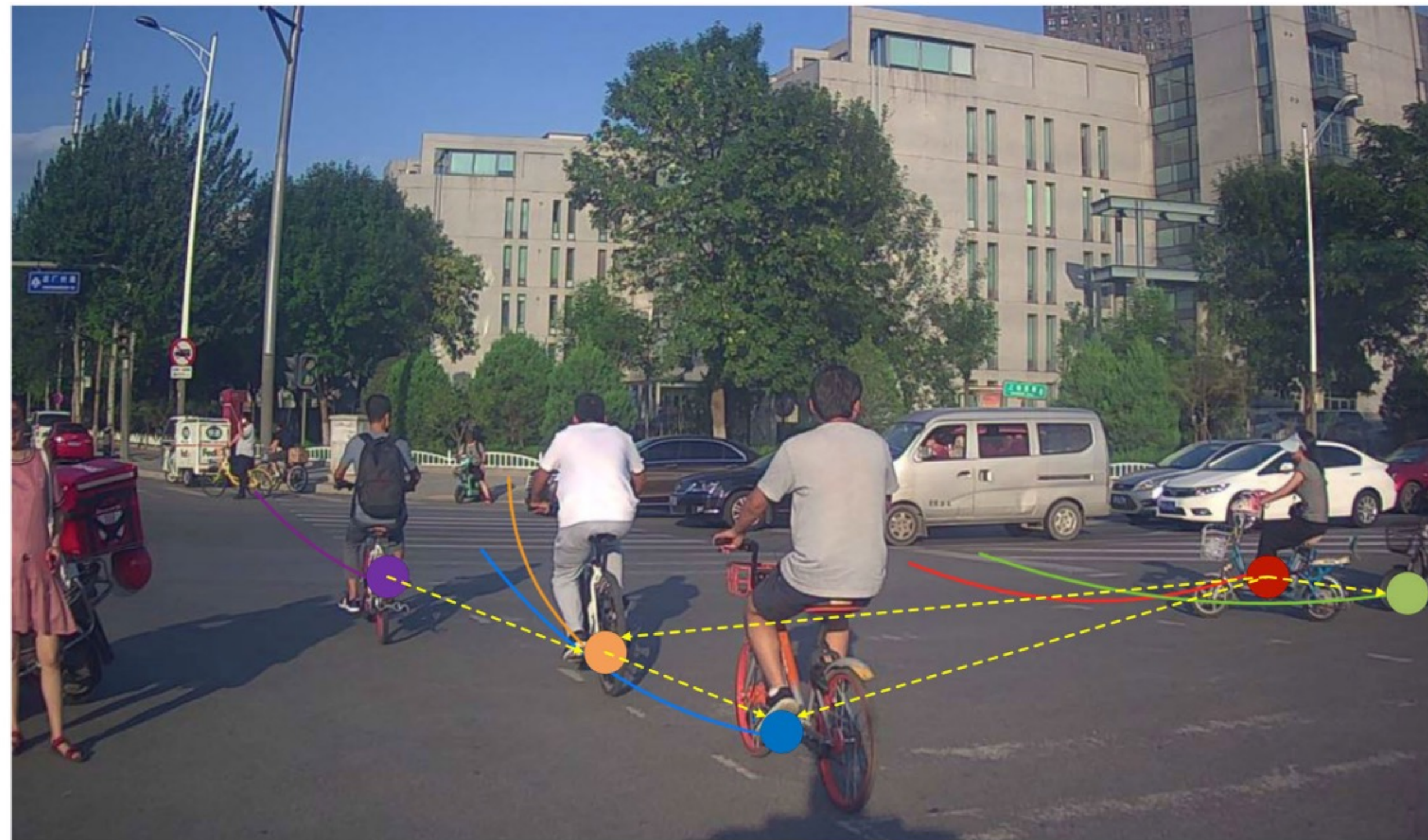
Fig. 1. Illustrations of trajectory prediction with captured social interactions. Dots of different colors represent the graph nodes that encode the motion patterns of different traffic-agents. The dashed lines represent the graph edges that capture the social interactions among different traffic-agents. The solid lines represent their future trajectories.
