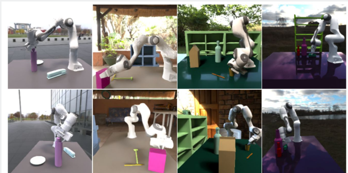
Figure 6: Sample scenes from the kitchen dataset. The top and bottom rows show two different views. SORNet can leverage additional views to improve performance, but does not require multiple views.
