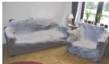
Figure 1. Mesh R-CNN takes an input image, predicts object instances in that image and infers their 3D shape. To capture diversity in geometries and topologies, it first predicts coarse voxels which are refined for accurate mesh predictions.
