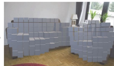
Figure 1. Mesh R-CNN takes an input image, predicts object instances in that image and infers their 3D shape. To capture diversity in geometries and topologies, it first predicts coarse voxels which are refined for accurate mesh predictions.
