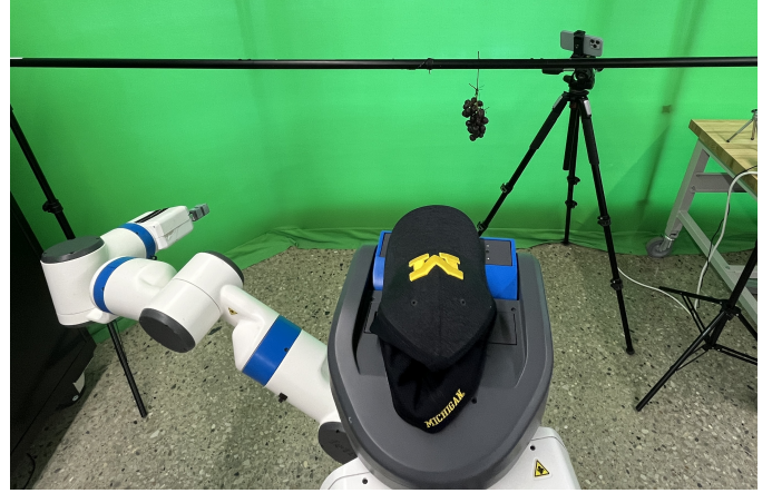
Fig. 4: Lab experiment setup. The grapes were suspended from a rod in front of the robot's view.
