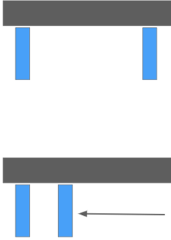
Fig. 3. Simple 1 DoF parallel gripper used in trials
